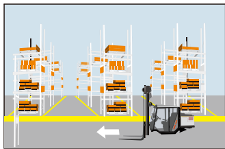
With sufficient ambient light, the sensor does not switch on the lamp.
